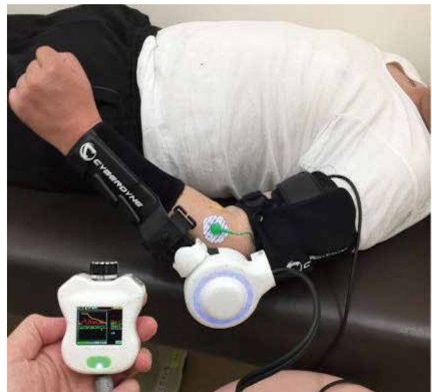
Fig 2. The single-joint Hybrid Assistive Limb(HAL-SJ). The controller showing the Bioelectrical signals.
